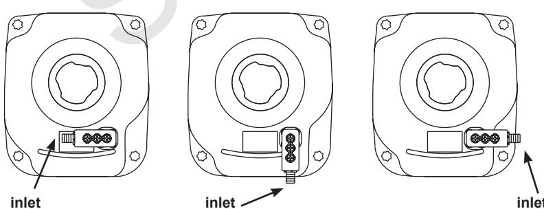
With the multiple inlet adapter, up to 4 condensate lines can be connected directly to the KCF unit.
